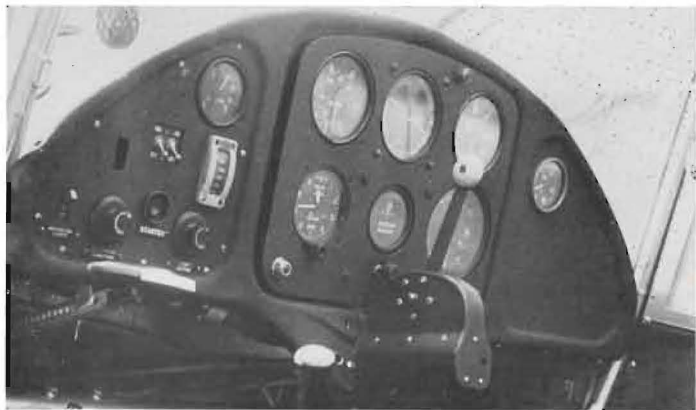
The instrument panel of the Auster Mk. 5D is now changed by the introduction of a new type of throttle control
