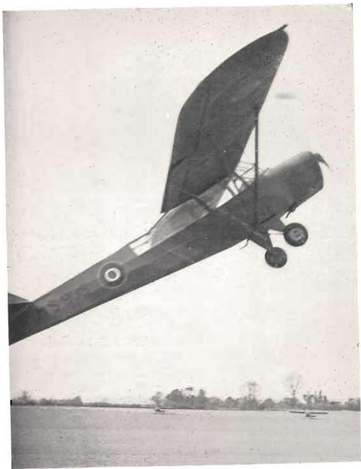
The Auster Mk. 5 in its original Service condition. The spectacular take-off portrayed in this photograph is one which usually captures the interest of visitors to Rearsby. Note the flaps in the take-off position.
